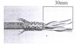
Strip approximately 30mm of the cable jacket, and separate to 4 pair each.
